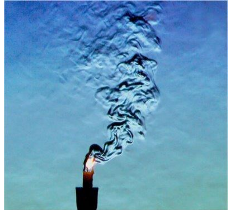
Schlieren image of a the thermal plume of a burning candle
